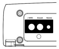
The G1700's "+12VDC" and "Ground" connections are designed to accept 4 AWG power wire. 4 AWG is a minimum power wire size for this amplifier.
